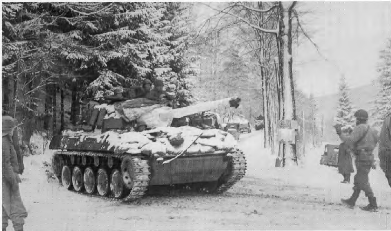
Winter in the Bulge. A snow covered M18 negotiates a narrow hairpin turn in the bitter cold of the Ardennes. Sandbags cover the thin glacis for added protection and a white sheet has been wrapped around the long gun tube to help blend with the snow when the TD reaches a firing position. US Army Photo SC 199435
