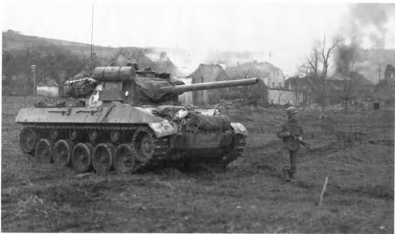
A Third Army Hellcat waits near a burning German village while a GI cautiously checks for mines. Note the usual cluttered stowage, stripped aiming stakes and battered condition of the flimsy front fenders. The detachable co-drivers' windshield has been discarded, and its square rack on the front side of the turret now holds a jerry can and a canteen cup. The USA number is 401453589. US Army Photo SC 201509
