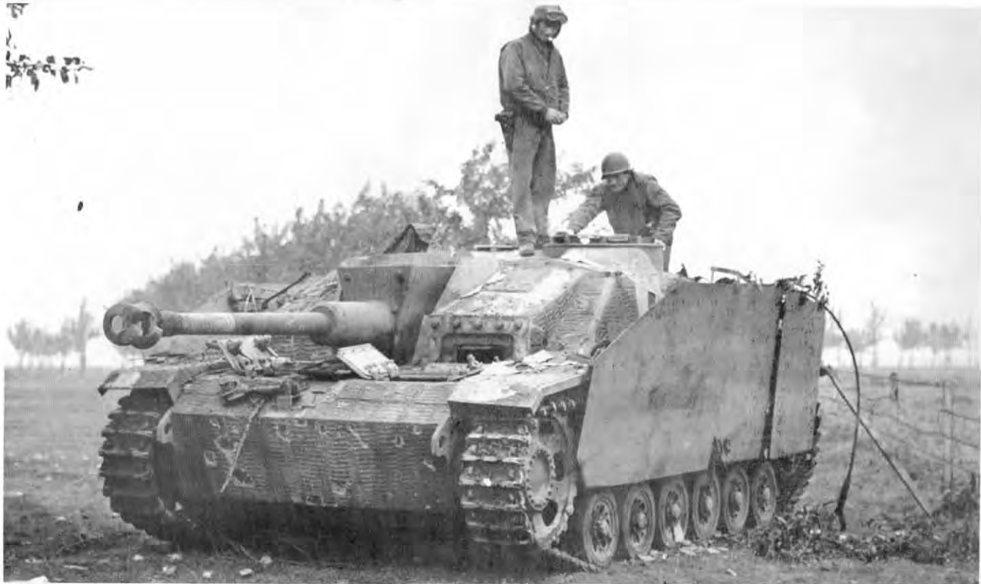
The German counterpart to the American tank destroyer featured a fully-armored fighting compartment and a low-silhouette in place of a turret. Typical of a number of different types of self-propelled (SP) guns employed in the ETO, the Sturmgeschütz III . was armed with the same 75mm gun as the Panzer IV . Camouflaged SPs were frequent opponents of the 4th Armored Division's advance.
