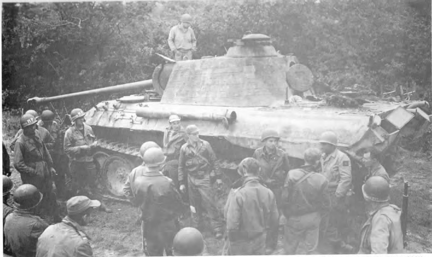
A well-balanced combination of armor, firepower and speed, the 49-ton Panther was generally regarded as the best tank of World War II. Well-sloped armor and a more powerful, high velocity gun made the Panther more formidable than the well-known Tiger . In this picture, a knocked-out Panther is being shown to correspondents and fighter pilots against the background of a Normandy hedgerow. U.S. Army Photo SC 191727.
