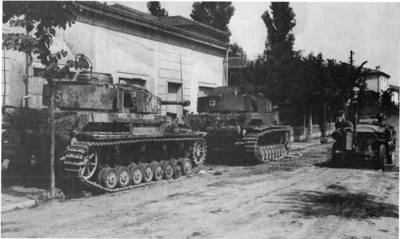
Mainstay of the Wehrmacht for most of the war, the Panzerkampfwagen IV , equipped at least one battalion of each Panzer-Regiment in 1944. Thin, detachable armor skirts on the sides of the hull (missing here) and turret provided spaced armor protection against American bazookas. Unless fighting from a dug-in, hull defilade defensive position, the Panzer IV could be defeated at medium ranges. U.S. Army Photo SC 191848.
