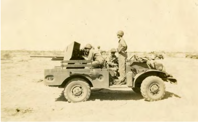
[Figure 4] M6 GMC, a ¾ ton weapon carrier. It was a poor platform. This is a picture of a unit from the 773 rd TDB training at Camp Young, California, 1942 (Spiess Jr. Collection, Jackson Barracks).
