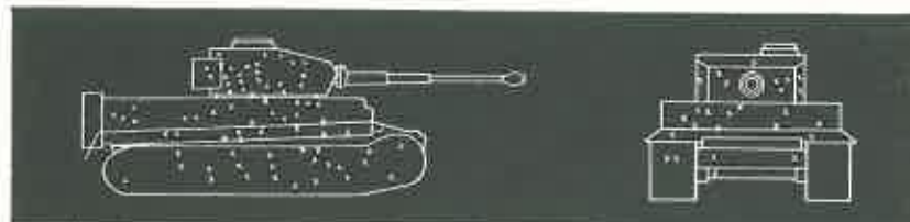
Figure 30. SITE OF HITS ON GERMAN MARK V AND VI TANKS.
