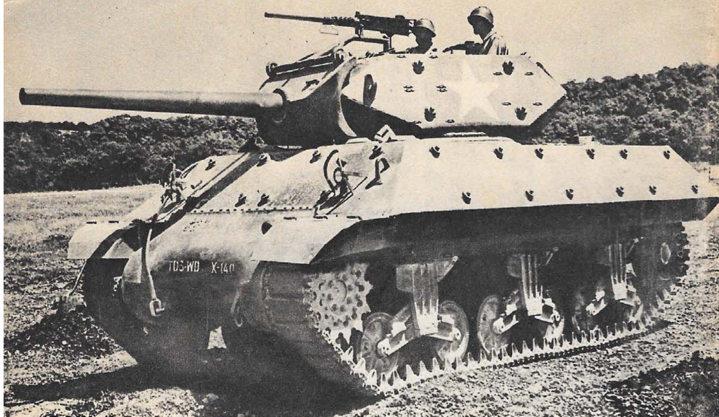
The Tank Destroyer M-10. The 3" gun and the 50 caliber machine gun spell trouble for the enemy.
