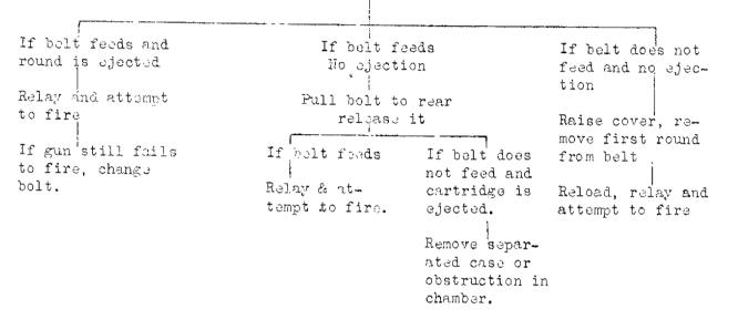
FOTE: This chart will not determine or locate broken parts, except in firing mechanism.
