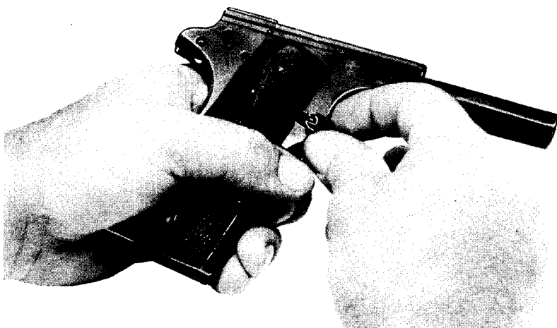
Figure 46. Disassembling old design magazine catch from receiver.
