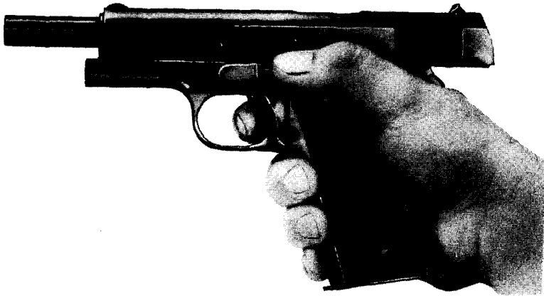
Figure 13. Pistol M1911A1, slide fully back, slide stop engaged, finger squeezing trigger, thumb releasing slide, hammer back.
