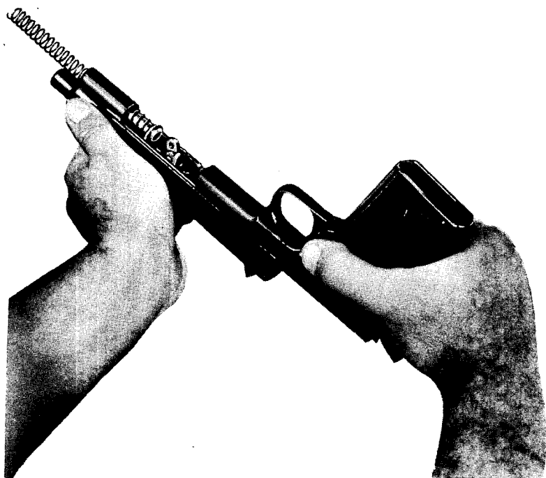
Figure 59. Installing slide group on receiver group, barrel link tilted forward.
