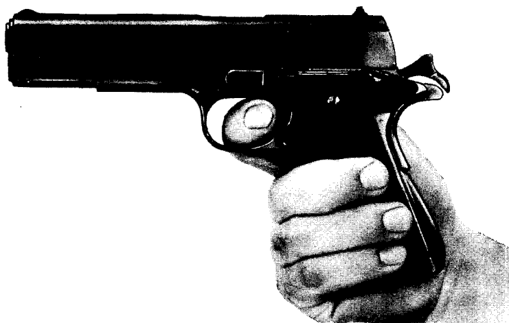
Figure 9. Pistol M1911A1, hammer cocked, grip safety not depressed, finger squeezing trigger.
