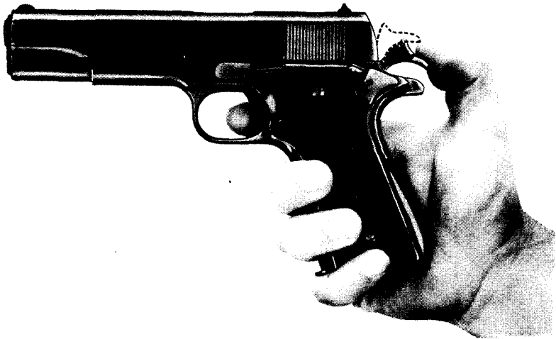
Figure 11. Pistol M1911A1, hammer back nearly to full cock position, thumb slipping off hammer.
