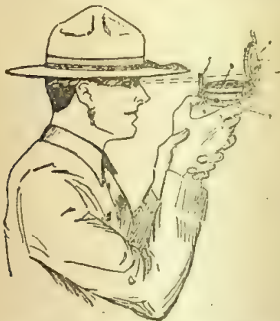
FIGURE 58.—Prismatic compass, showing compass open and in position for measuring azimuth in daylight.
