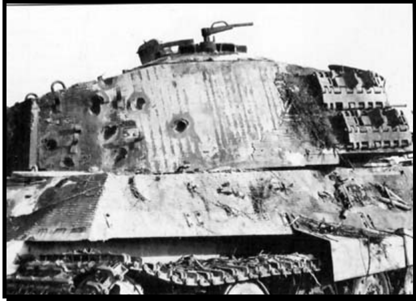
A Tiger Mark VI damaged with a 3" anti-tank gun
