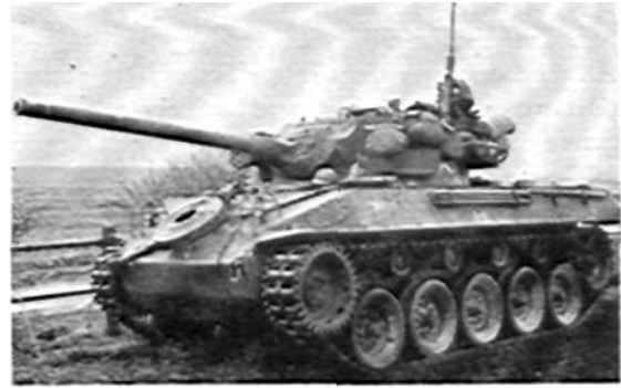
Mounting a 76-mm gun and a .50-cal. machine gun, the M18 tank destroyer has a road speed of 55 mph. Its turret has 360° traverse, both hand- and power-operated.
