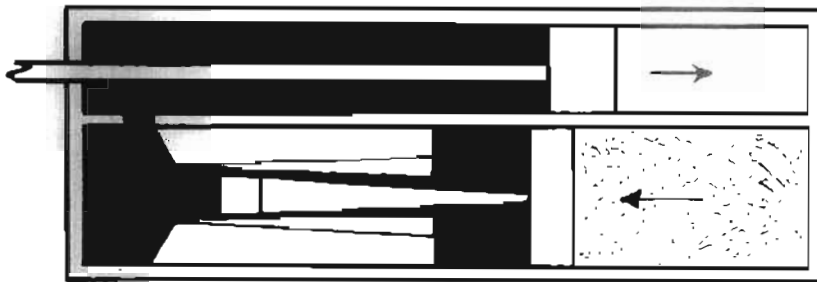
DIAPHRAGM MOVES TO REAR - TAPERED CONTROL ROD GRADUALLY CLOSSES TAPERED GROOVES
